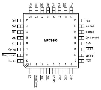
Figure 2. 32-Lead Pinout (Top View)
