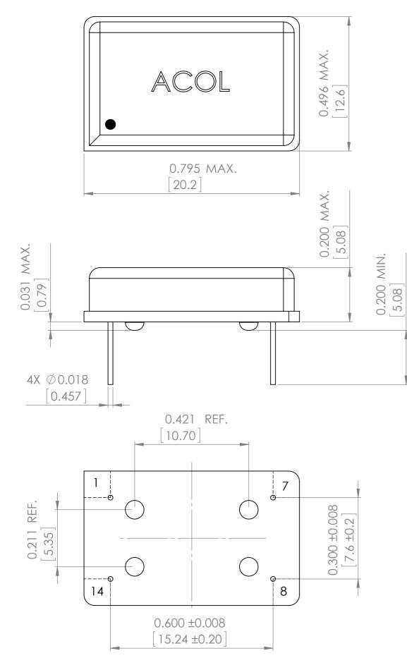
The height of the package vary depending on the frequency >100MHz. Please contact ABRACON for the height information for F>100MHz.
