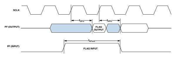
Figure 9. Programmable Flags Cycle Timing
