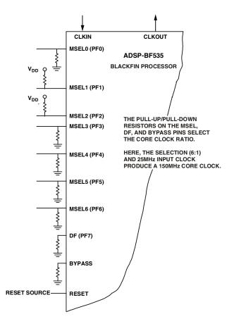
Figure 7. Clock Ratio Example
