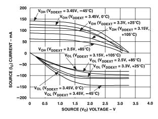
Figure 21. PCI\_REQ Output Drive Current
