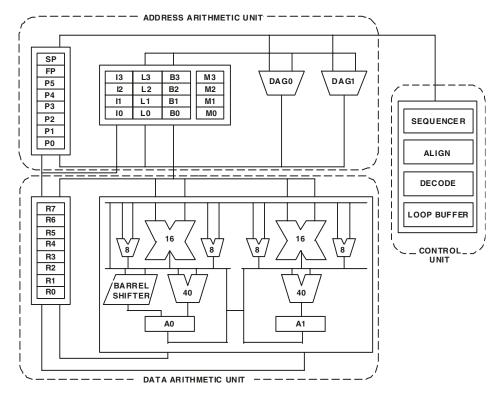
Figure 1. Processor Core
