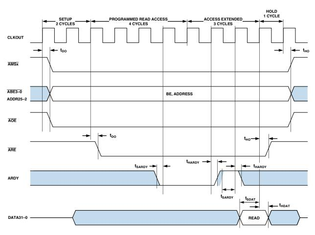
Figure 12. Asynchronous Memory Read Cycle Timing
