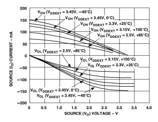
Figure 19. Output Drive Current
