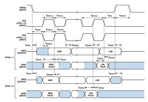
Figure 16. Serial Peripheral Interface (SPI) Port-Slave Timing
