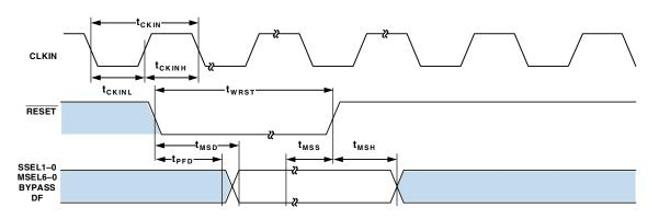
Figure 8. Clock and Reset Timing
