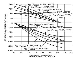
Figure 20. PCI 33 MHz Output Drive Current
