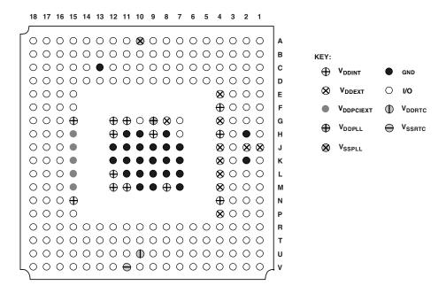
Figure 26. 260-Ball Metric PBGA Pin Configuration (Bottom View)
