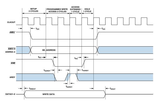
Figure 11. Asynchronous Memory Write Cycle Timing
