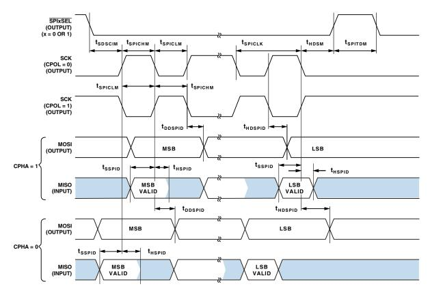
Figure 15. Serial Peripheral Interface (SPI) Port-Master Timing
