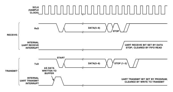
Figure 17. UART Port-Receive and Transmit Timing
