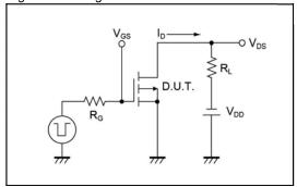
Fig.2-1 Gate Charge Measurement Circuit
