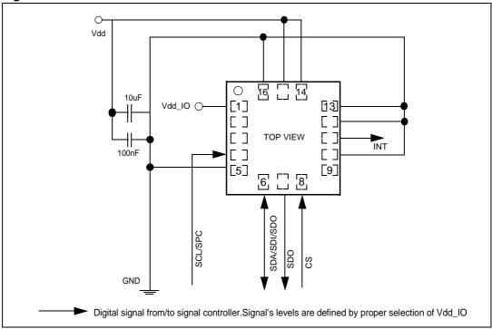
The device core is supplied through Vdd line while the I/O pads are supplied through Vdd\_IO line. Power supply decoupling capacitors (100 nF ceramic, 10 µF AI) should be placed as near as possible to the pin 14 of the device (common design practice).
