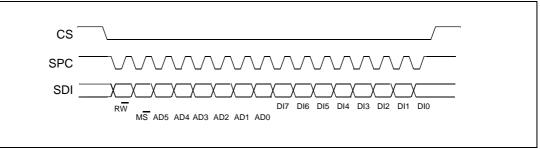
The SPI Write command is performed with 16 clock pulses. Multiple byte write command is performed adding blocks of 8 clock pulses at the previous one.
