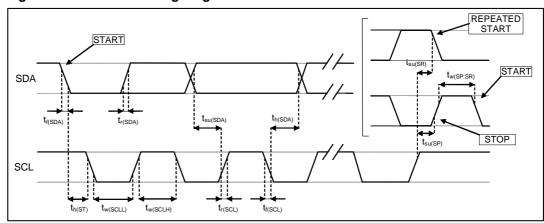
4. Measurement points are done at 0.2·Vdd\_IO and 0.8·Vdd\_IO, for both ports
