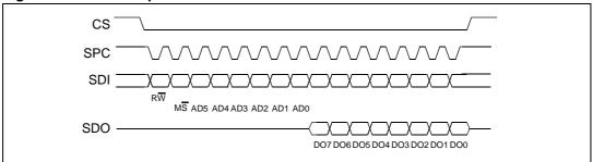
The SPI read command is performed with 16 clock pulses. Multiple byte read command is performed adding blocks of 8 clock pulses at the previous one.
