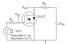
Fig. 10a - Switching Time Test Circuit
