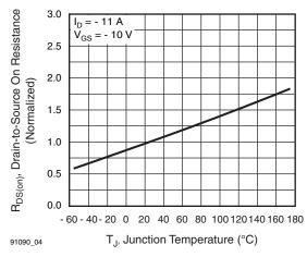
Fig. 4 - Normalized On-Resistance vs. Temperature
