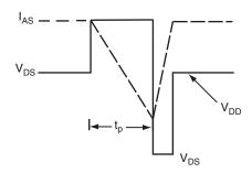
Fig. 12b - Unclamped Inductive Waveforms
