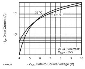
Fig. 3 - Typical Transfer Characteristics
