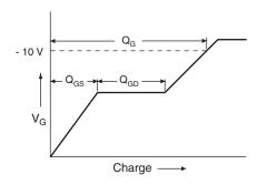
Fig. 13a - Basic Gate Charge Waveform
