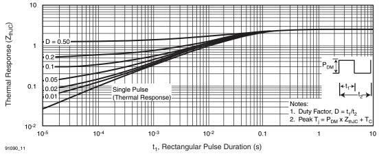
Fig. 11 - Maximum Effective Transient Thermal Impedance, Junction-to-Case
