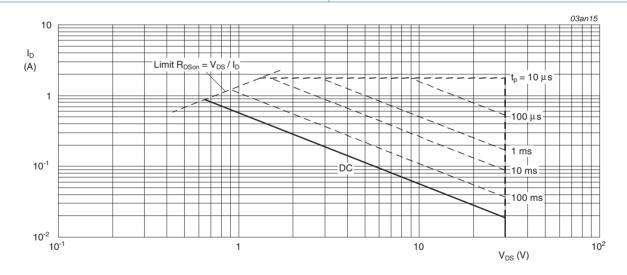
$T_{SP} = 25$  °C;  $I_{DM}$  is single pulse;  $V_{GS} = 4.5V$
