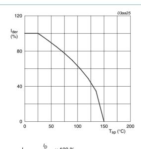
$I_{der} = \frac{I_D}{I_{D(25\,^{\circ}\text{C})}} \times 100 \%$
