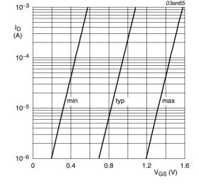
$$T_j = 25 \,^{\circ}C; V_{DS} = 5V$$
