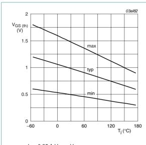
$I_D = 0.25 \, A; V_{DS} = V_{GS}$
