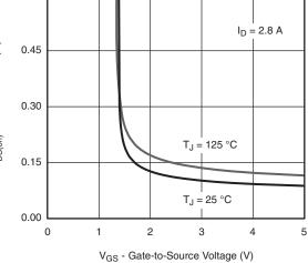
On-Resistance vs. Gate-to-Source Voltage
