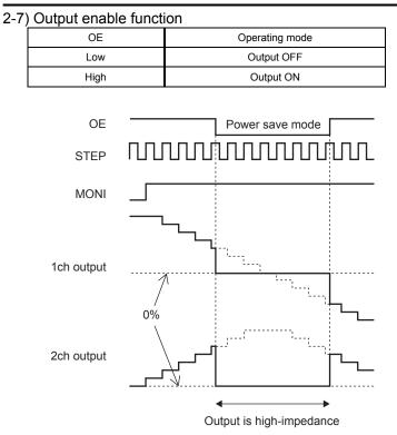
When the OE pin is set Low, the output is forced OFF and goes to high impedance.
