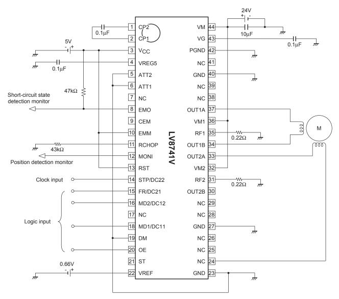
The setting conditions for the above circuit diagram example are as follows :
