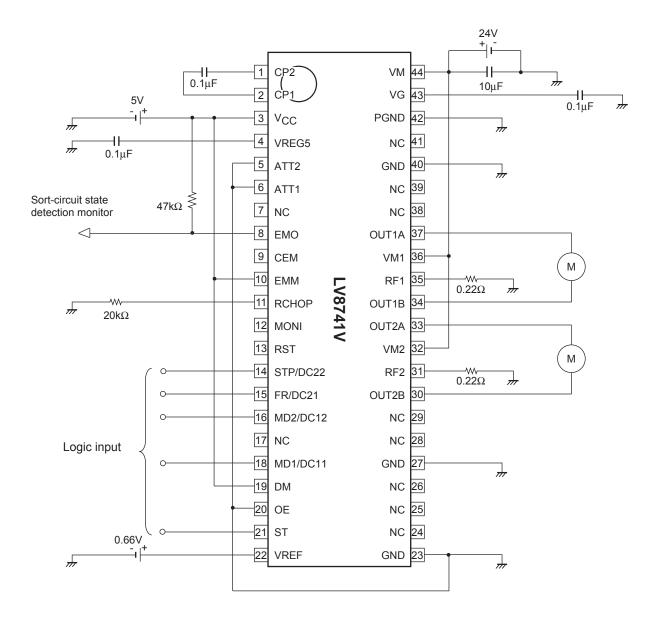
The setting conditions for the above circuit diagram example are as follows : At the time of VREF = 0.66V, setting electric current ratio 100% [(ATT1, ATT2) =(L,L)], RF resistance 0.22 $\Omega$ , the current limit value is as follows .
