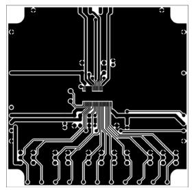
L1 : Copper wiring pattern diagram
