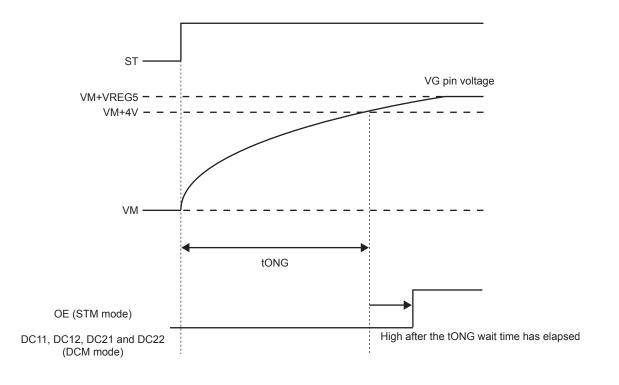
VG Pin Voltage Schematic View
