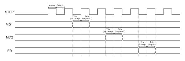
TstepH/TstepL : Clock H/L pulse width (min 500ns) Tds : Data set-up time (min 500ns) Tdh : Data hold time (min 500ns)
