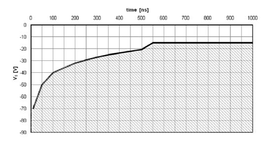
Figure 28: Negative V<sub>S</sub> transient SOA for AUIRS2332J
