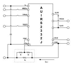
Figure 9: Programming the over-current protection
