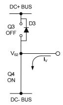
Figure 23: D3 conducting
