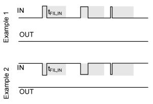
Figure 14: Noise rejecting input filters
