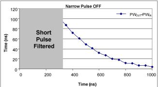
Figure 16: Difference between the input pulse and the output pulse
