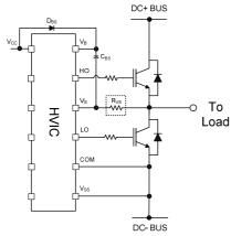
Figure 36: V<sub>S</sub> resistor
