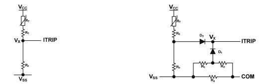
Figure 10: Programming over-temperature protection Figure 11: Using over-current protection and over-temperature protection
