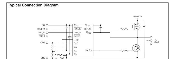
(Refer to Lead Assignments for correct pin configuration). This/These diagram(s) show electrical connections only. Please refer to our Application Notes and Design Tips for proper circuit board layout.
