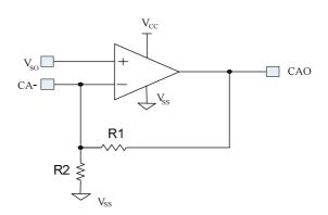
Figure 29: Current amplifier typical configuration
