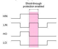
Figure 8: Illustration of shoot-through protection circuitry
