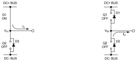
Figure 21: Q1 conducting
