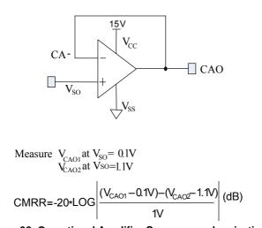
Figure 32: Operational Amplifier Common mode rejection measurement
