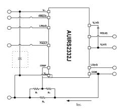
Figure 35: Supply capacitor
