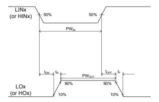
Figure 3: Switching time waveforms
