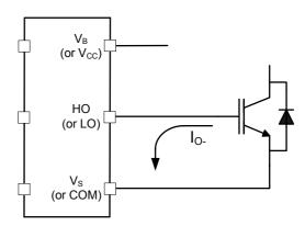
Figure 2: HVIC sinking current
