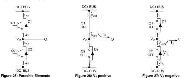
In a typical motor drive system, dV/dt is typically designed to be in the range of 3-5 V/ns. The negative  $V_S$  transient voltage can exceed this range during some events such as short circuit and over-current shutdown, when di/dt is greater than in normal operation.
