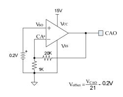
Figure 31: Operational Amplifier Input Offset Voltage measurement
