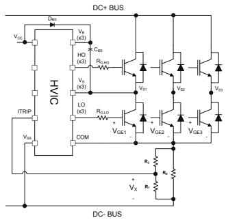
Figure 19: Separate V<sub>SS</sub> and VSO (COM) pins
