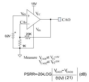
Figure 33: Operational Amplifier Power supply rejection measurement
