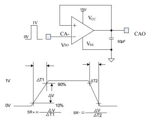
Figure 30: Operational Amplifier Slew rate measurement
