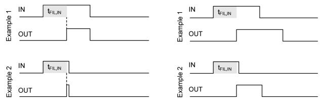
Figure 13: Advanced input filter
