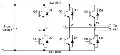
Figure 20: Three phase inverter
