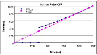
Figure 15: AUIRS2332J input filter characteristic
