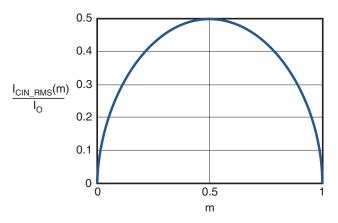
Figure 2. I<sub>CIN</sub> vs. Voltage Conversion Ratio
